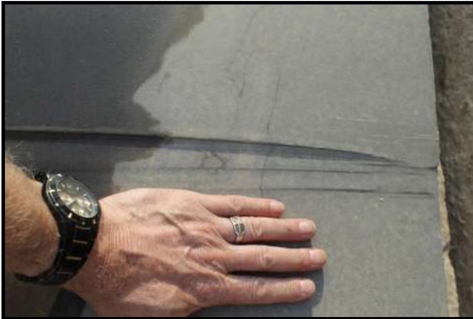
Evidence that the saw changed its cutting path
